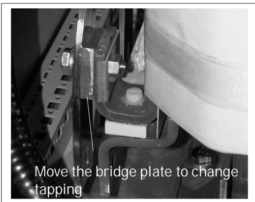
Figure 5-6. Input chokes tapping in FR13/14 units
